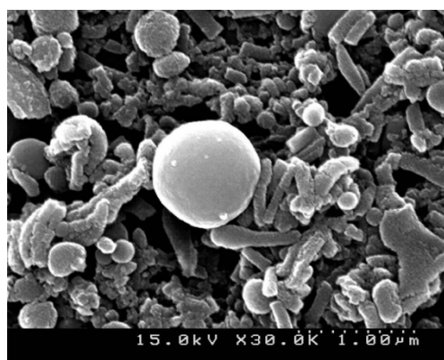
Figure 5 SEM image of poly(BVPCHMI-co-ST)
