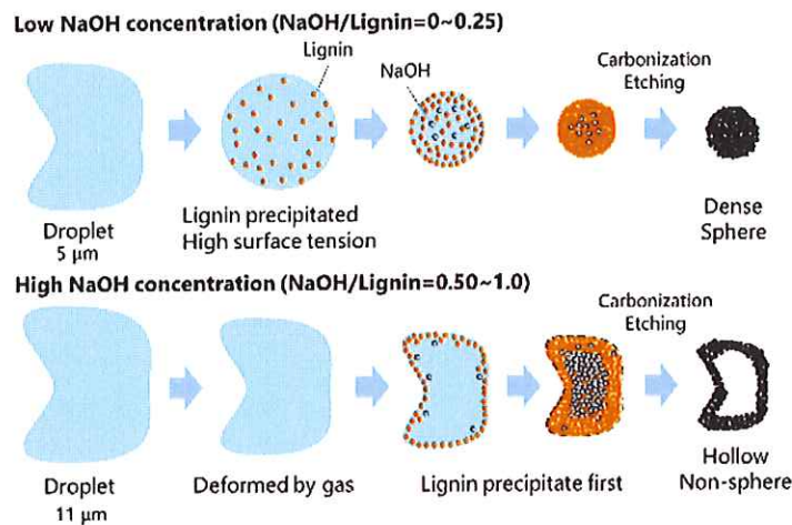
Fig. 5 Particle formation mechanism: (a) Low NaOH concentration, (b) High NaOH concentration
